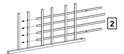
Insert two 63" vertical slats (part 6) through outer holes of center cross rails and into bottom cross rail. Insert two 66" vertical slats (part 7) through inner holes of center cross rails and into bottom cross rail.
