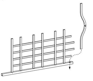
Insert top bent rail (part 5) through right post, inserting vertical slats into top bent rail.
