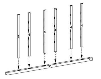
Lay out one right post (part 2). Starting at bottom, insert one bottom cross rail (part 3) and five center cross rails (part 4).
