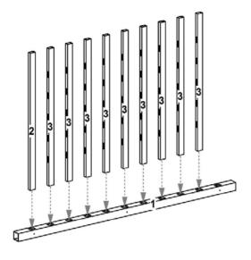
Lay out one post (part 1). Starting at one end, insert one top/bottom cross rail (part 2) and nine center cross rails (part 3).
