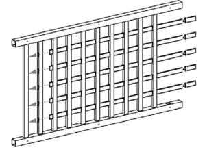
Insert vertical slats (part 4) through center cross rails and into bottom cross rail.
