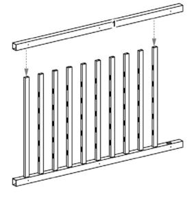
Slide remaining post (part 1) over corresponding cross rails.
