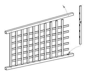
Separate top of posts just enough to insert remaining top/bottom rail (part 2).
