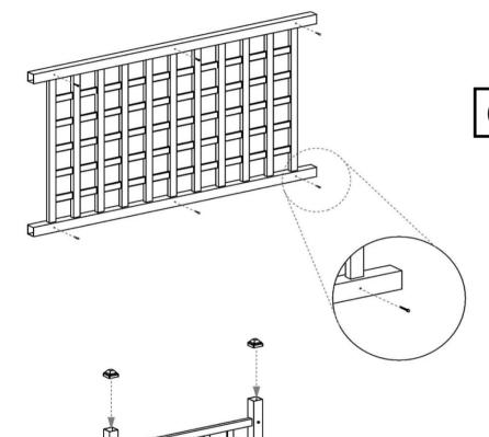
Using 1¼" painted screws, screw together trellis. Be sure that all parts are fully inserted into posts before securing.
