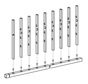
Lay out right post (part 2). Starting at bottom (flared end), insert bottom cross rail (part 4) and center cross rails (part 3).
