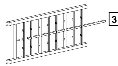
Insert 58" vertical rail (part 5) through center hole of cross rails.
