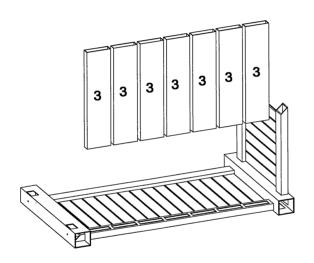
2 Insert seven % x 3 x 13¼" bottom rails (part 3) into holes of planter side WITH posts.
