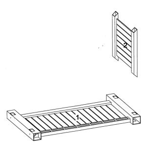
Insert ends of on planter side WITHOUT posts (part 2) into right post of planter side WITH posts (part 1).
