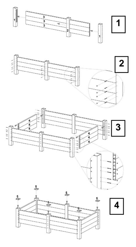
Insert three 1 ½"x 5 ½"x 94" rails (part 3) through one 4'x 4"x 24" line post (part 2). Insert ends of 94" rails into two 4"x 4" 24" corner posts (parts 1). Slide line post to center of rail.
