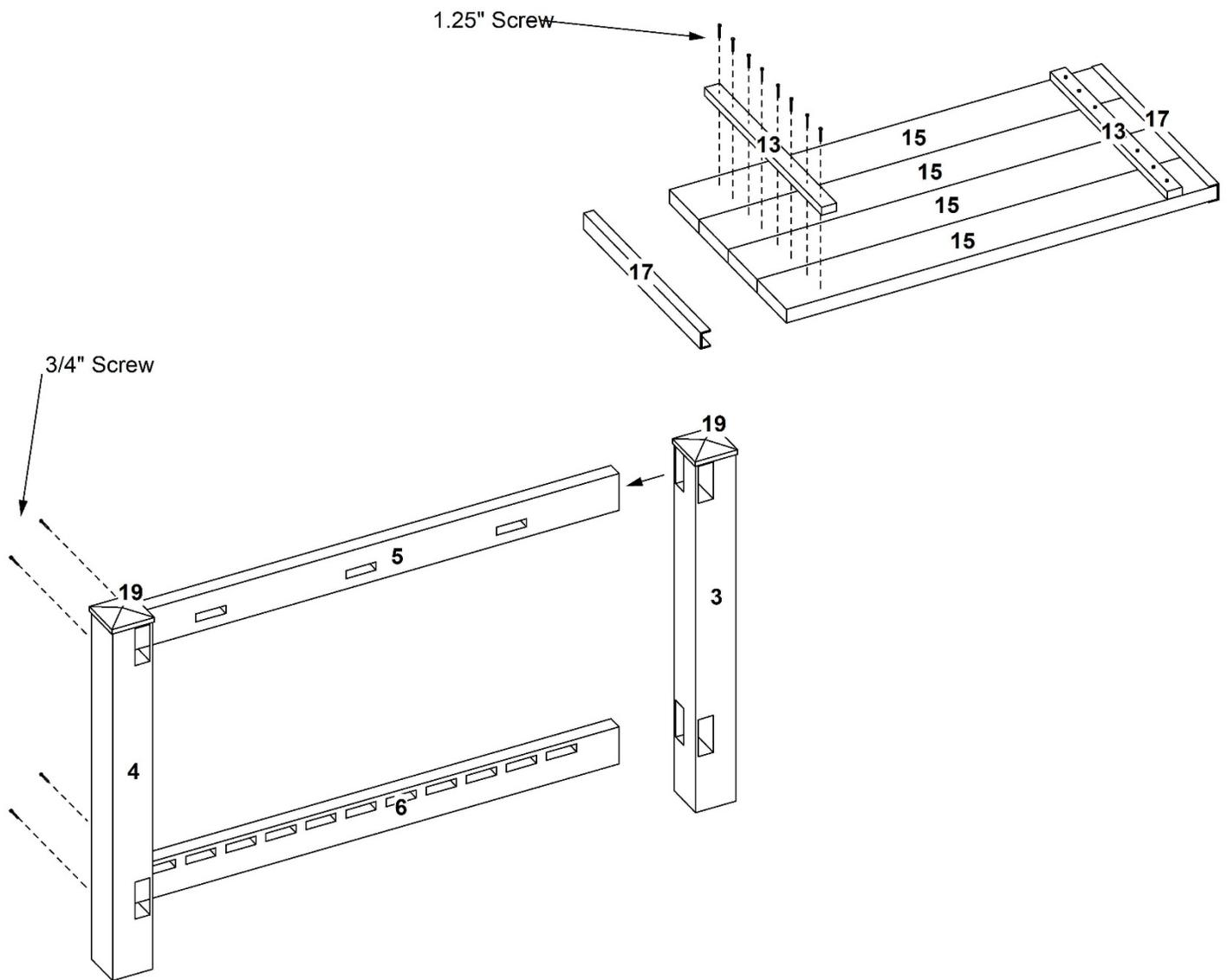
Insert one 51½" table rail (part 5) into 38" front right post (part 4). Insert one 51½" shelf rail (part 6) into 38" front right post. Insert free ends of table and shelf rail into 38" back left post (part 3). Using four ¾" screws per post, screw together potting bench front panel. Be sure all parts are fully inserted into posts before securing. Using included super glue tube, glue 4" sq. flat post cap (part 19) onto top of each post.
