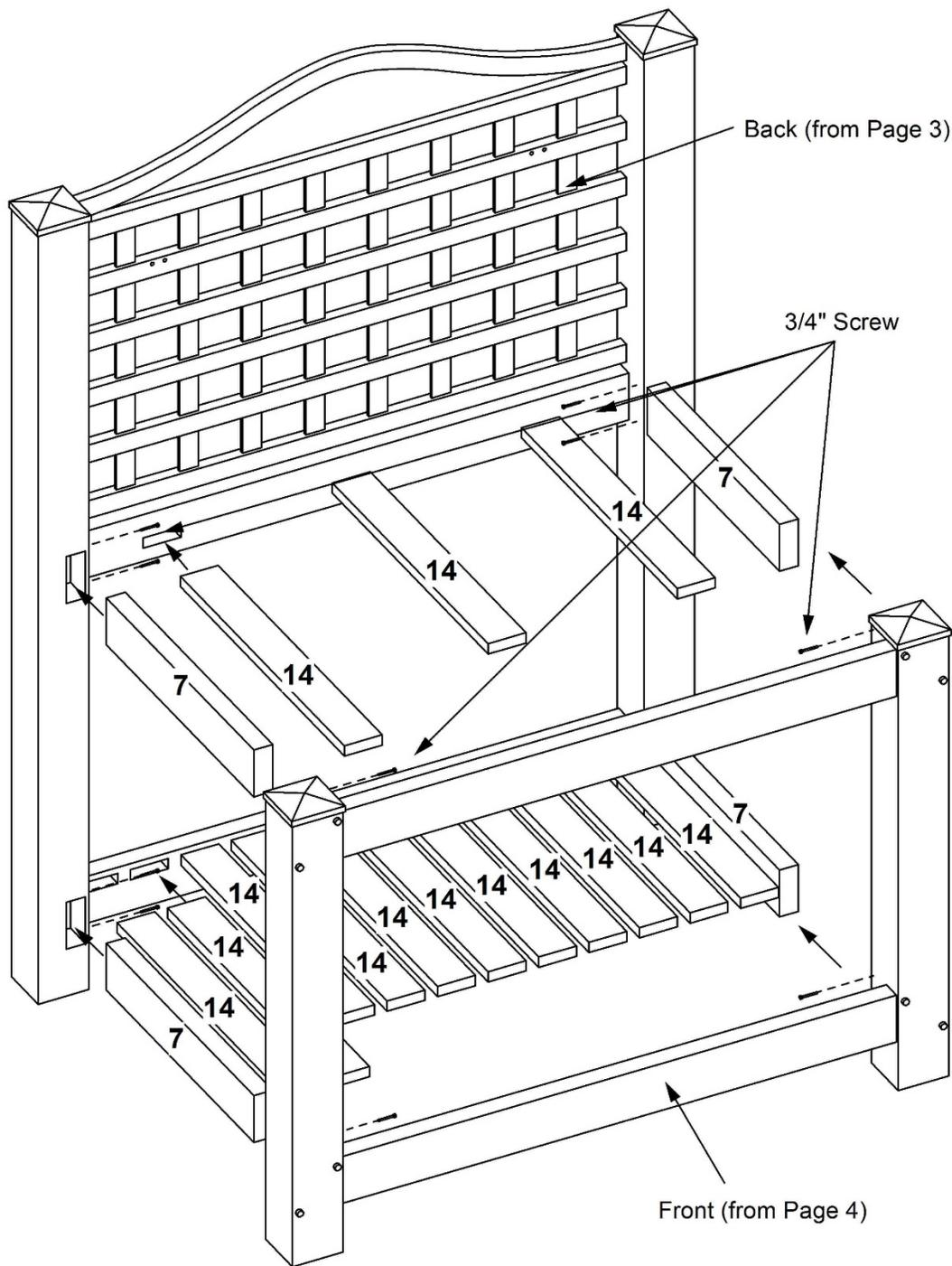
Insert four 22" side rails (part 7) into posts of potting bench pack panel (from page 3). Insert three 24½" table/shelf rails into table rail of back panel. Insert eleven table/shelf rails into shelf rail of back panel. Insert free ends of side rails and table/shelf rails into corresponding holes of potting bench front panel (from page 4). Using four ¾" screws per post, fasten together potting bench. Be sure all parts are fully inserted before securing.
