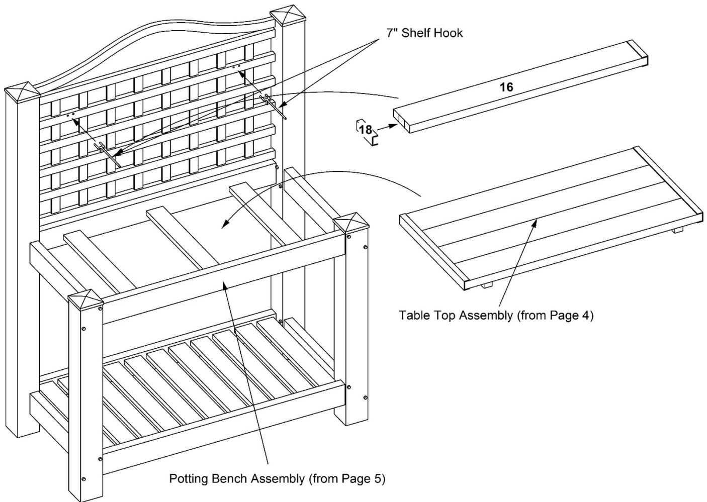
Apply glue to inside edges of 5½" shelf end cap. Press end cap onto ends of 43" shelf rail (part 16) (DO NOT slide from end). Insert two 7" shelf hooks from hardware packet into pre-drilled holes and place shelf on top of hooks.
