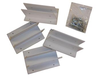
Set assembled bench in desired location. Slide the two 5 <sup>1</sup>/<sub>2</sub>" brackets under back legs of bench and the two angled brackets under the front legs. With 1 <sup>1</sup>/<sub>4</sub>" screws fasten brackets to pier or deck. With bench setting on brackets, use the <sup>1</sup>/<sub>4</sub>" drill bit to drill holes through bench legs, using the predrilled holes in brackets as your guide. Fasten bench to brackets using 2 <sup>1</sup>/<sub>4</sub>" bolts, washers and nylock nuts.
