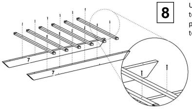
Using 1¼" screws, screw six of eight arbor top cross rails with caps to arbor top panels (part 7). Do not attach end arbor top cross rails at this time
