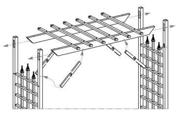
Insert one end of each 18" corner brace (part 9) into routed hole on bottom of arbor top rails. Insert ends of arbor top rails through holes at top of each post of arbor panels, inserting free ends of corner braces into other routed holes in posts.
