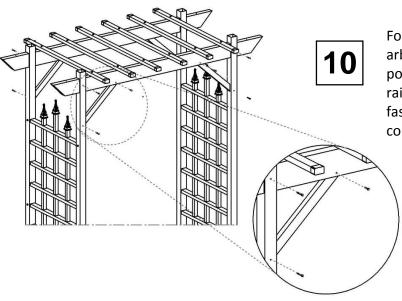
For each post, measure from tip of each arbor top rail to outside of post and move post so it is 9 inches from end of arbor top rails. Using three 1¼" screws per post, fasten together post, arbor top rail and corner brace.
