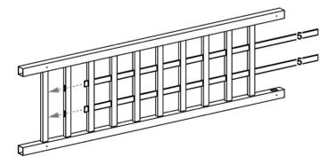
Insert vertical slats (part 5) through center cross rails and into bottom cross rail.
