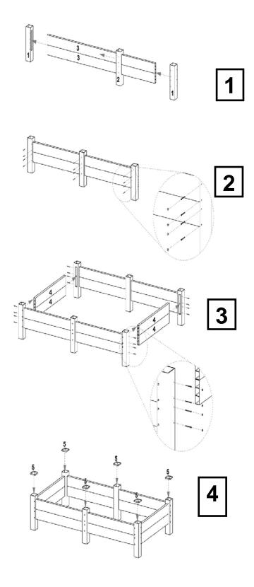
Insert two 1 ½"x5 ½"x 96" rails (part 3) through one 4"x 4"x 19" line post (part 2). Insert ends of 96" rails into two 4"x 4"x19" corner posts (part 1). Slide line
