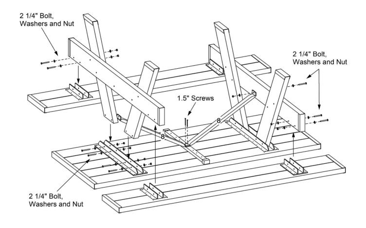
Insert one cross brace / leg assembly into brackets on underside of table top with cross brace closest to table end. Using four 2½" bolts, washers and nuts, fasten assembly to table top. Repeat with second cross brace / leg assembly for opposite end of table.
